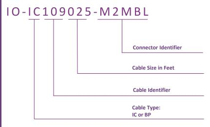
\* Cables with right angle connectors are designated by "-R" for one right angle connector, and a "-2R" for 2 right angle connectors.
